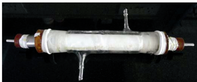
Figure 8. Spiral wound membrane (CD) module.
