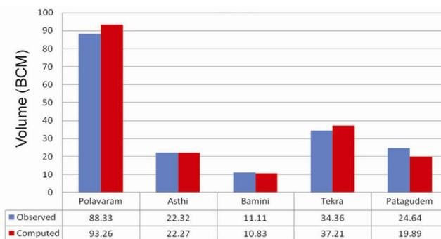
Figure 5. Observed and calibrated run-off (mean of 18 years) at various gauge stations.
