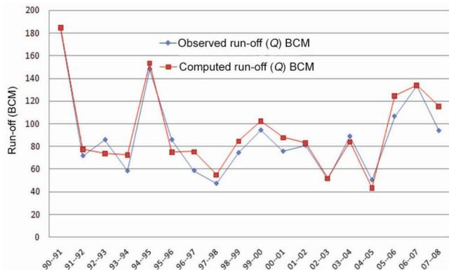
Figure 4. Observed and calibrated run-off at Polavaram during 18 years (1990–91 to 2007–08).
