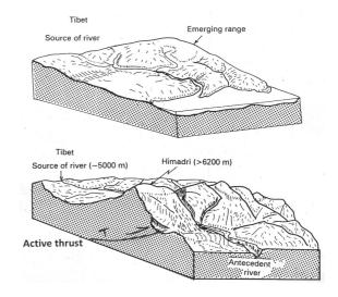
Figure 6. Evolution of a gorge as the hill gradually rose due to movement on an active thrust plane.
