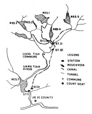
**Figure 10.** Multi-purpose cascade development scheme in which small rivers, rivulets and streams are utilized for storing water (after Naibo<sup>30</sup>).
