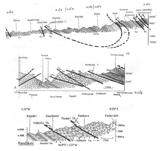
**Figure 3.** Sections across the MCT zone in Uttarakhand Himalaya showing active thrust planes (thick line) along the valleys of the Kali, Alaknanda and Mandakini rivers. Note how the Lesser Himalayan rock assemblages slide under the Great Himalaya, even as the rock piles of the latter advance southwards over the former (Lesser Himalayan assemblages) (after Valdiya<sup>1,5</sup>).
