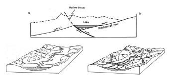
**Figure 7.** Due to uplift on a fault/thrust plane and heaving up of the ground, the gradient of the river bed decreases, causing deposition of its sedimentary load. Subsequent spurts of uplift are responsible for the formation of many levels of terraces – the evolution of stepped terraces. (Diagrammatic sketches after Valdiya<sup>5</sup>.)
