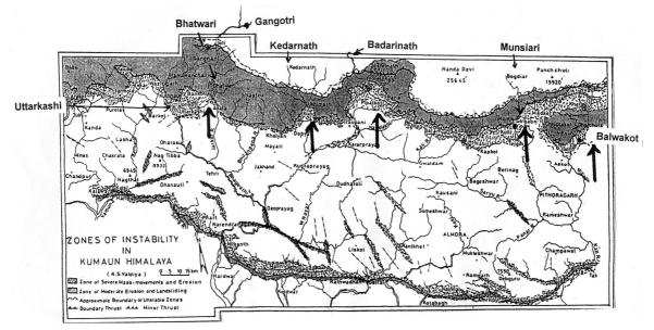
**Figure 8.** The MCT zone, characterized by active thrusts, endemic landslides and recurrent earthquakes, is a belt of unstable slopes vulnerable to seismic shocks, battering of rains and human activities (after Valdiya<sup>23</sup>).
