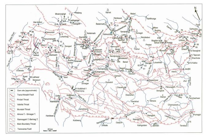
**Figure 1.** Structural map of Uttarakhand showing locations of big dams (height >25 m) in existence, under construction and those planned. The positions of dams are approximate. The structural elements comprise major thrusts and transverse (tear) fault dissecting the land. (Map after Valdiya<sup>1</sup> and location of dams after Thakkar<sup>2</sup> and Patni (pers. commun., 2013)).
