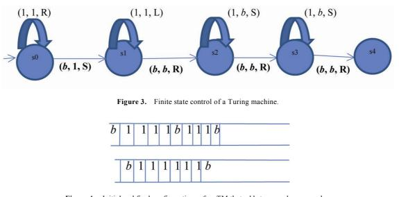
Figure 4. Initial and final configurations of an TM that adds two numbers, *m* and *n*.
