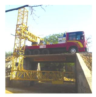
Figure 2. Mobile bridge inspection unit.
