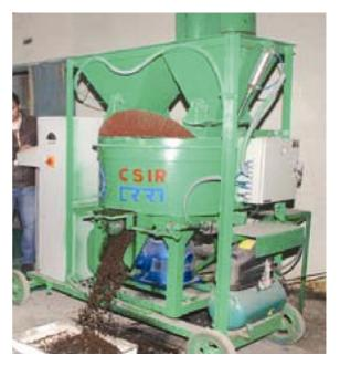
Figure 3. Portable pothole repair machine.
