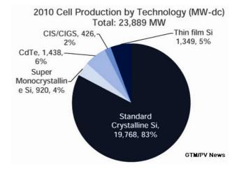
Figure 1. Break-up of global photovoltaic technologies.
