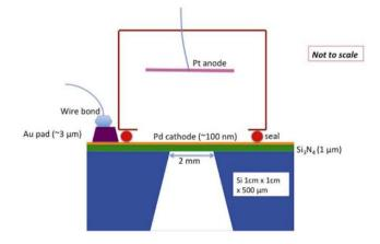
Figure 2. Schematic of membrane experiment.
