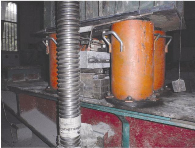
**Figure 2.** Loading device of three-point bending test.
