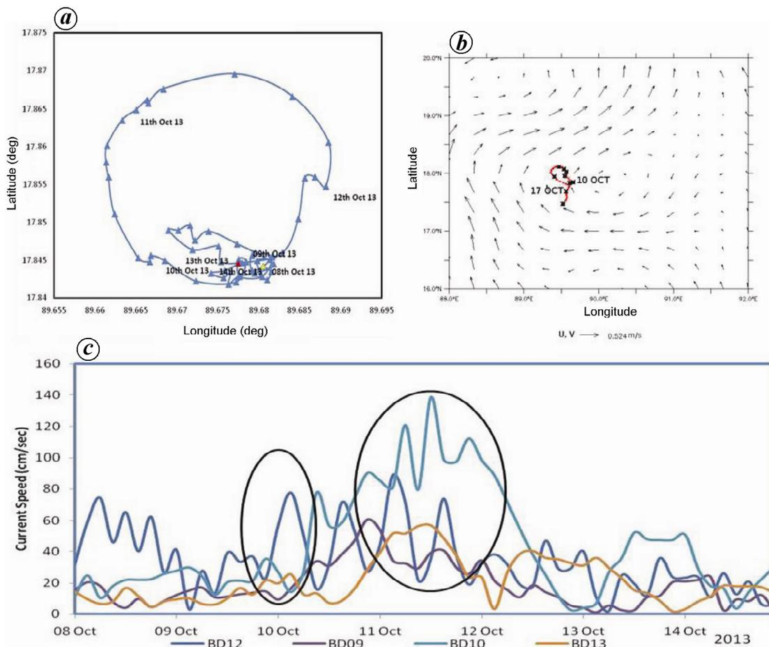
**Figure 6.** *a*, The drift of the buoy BD09\_18N/89E with the surface current following a clockwise path. *b*, Progressive position vector drawn based on the surface current data obtained from BD09\_18N/89E plotted against the OSCAR surface current for 11 October. *c*, Increase in current speed as recorded by the OMNI buoys in BoB.
