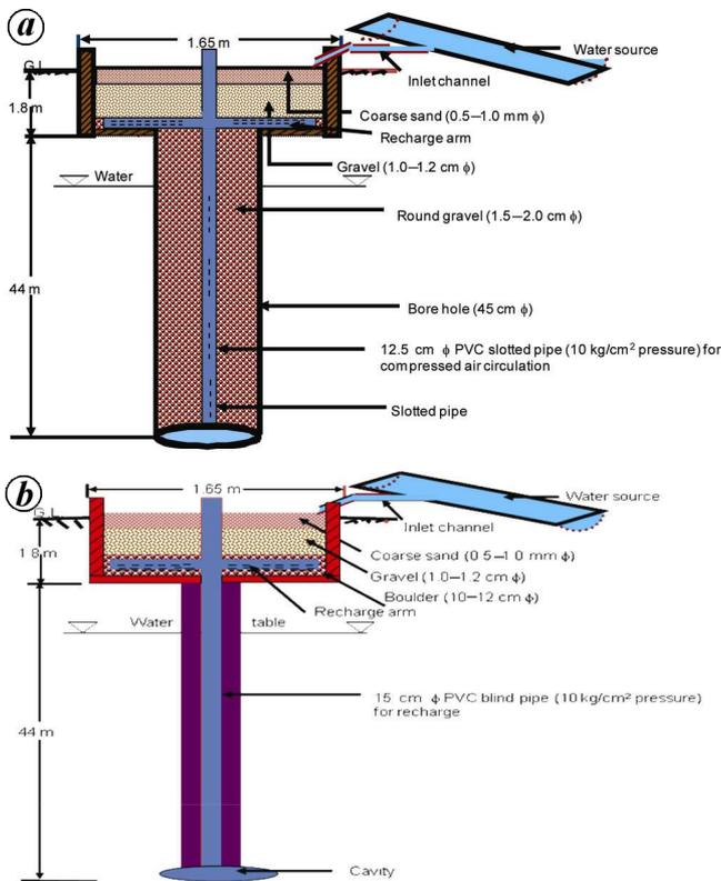
Figure 1. a, Schematic diagram of a recharge shaft. b, Schematic diagram of a recharge cavity.
