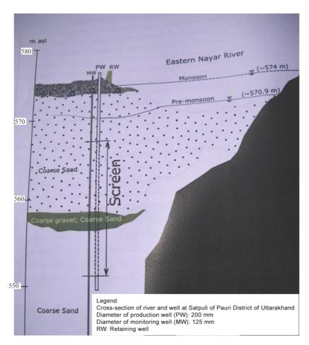
**Figure 2.** A schematic cross-sectional diagram of RBF location at Satpuli near East Nayar river in Pauri district of Uttarakhand<sup>39,40</sup>.
