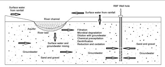
Figure 1. Modified general scheme of RBF<sup>2</sup>.
