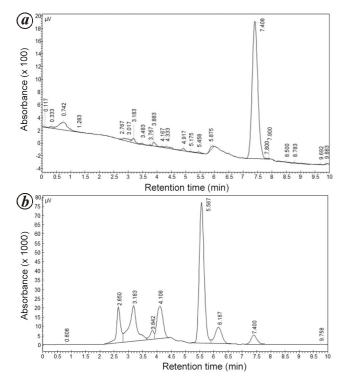
Figure 1. HPLC chromatograms of galanthamine authentic sample (*a*) and *Crinum* species bulb extract (*b*) detected using Innertsil C18 column and UV absorbance monitored at 288 nm utilizing methanol: 5 mM, (NH<sub>4</sub>)<sub>2</sub>HPO<sub>4</sub> (55:45) as mobile phase at a flow rate of 0.8 ml min<sup>-1</sup>.
