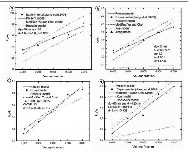
**Figure 3.** Effective thermal conductivity of carbon nanotube nanofluid with: *a*,  $d_p = 15$  nm,  $a_r = 100$  nm, d = 1.6 and n = 1.096; *b*,  $d_p = 15$  nm,  $a_r = 666-7$  nm, d = 1.6 and n = 1.051; *c*,  $d_p = 80$  nm,  $a_r = 18.8$  nm, d = 1.4 and n = 0.937; *d*,  $d_p = 80$  nm,  $a_r = 125$  nm, d = 1.4 and n = 0.928.
