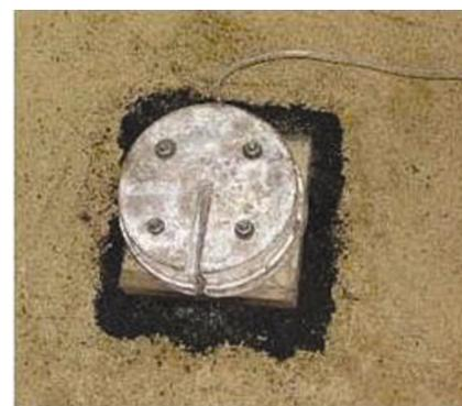
**Figure 5.** A view of the model footing (with surcharge load on top) resting on a base isolator consisting of 50% sand and 50% shredded rubber tyre.
