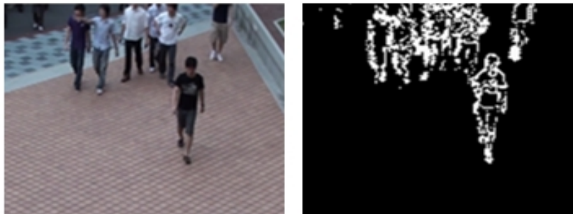
Figure 6. Obtaining the moving edges by subtracting consecutive images
