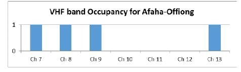
Fig 18: VHF band occupancy measurement for Afaha-Offiong.
