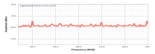
Fig 4: RSS amplitude against measured frequency points in the VHF band at Asong.
