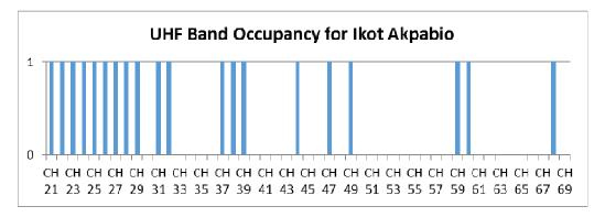
Fig 15: UHF band spectrum occupancy for Ikot Akpabio
