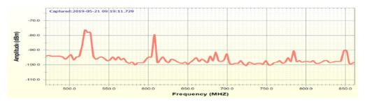
Fig 13: Amplitude versus frequency at the UHF band at Ikot Akpabio in Etinan LGA.
