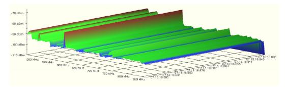
Fig 8: Waterfall imaging showing the RSS per frequency and time measured.
