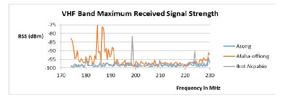
Fig 3 Maximum Received Signal strength on the VHF Band
