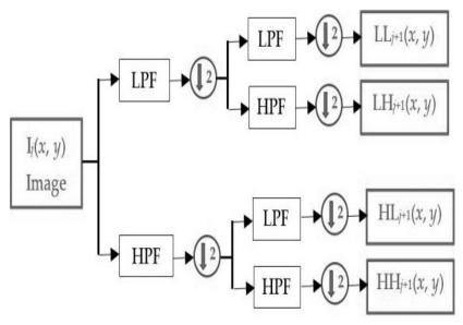
Fig 2. 2DWT of 'I' from level j to j + 1 produce sub-bands LLj+1, LHj+1, HLj+1, and HHj+1
