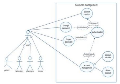
Fig 3. Use Case diagram for accounts management
