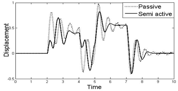
Fig. 18: Comparison of displacement at centre of gravity for passive and semi-active half car model.
