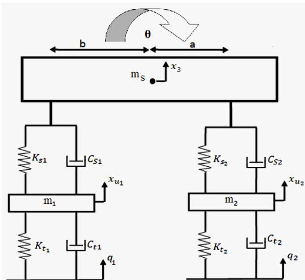
Fig. 13: Half car model for passive suspension system
