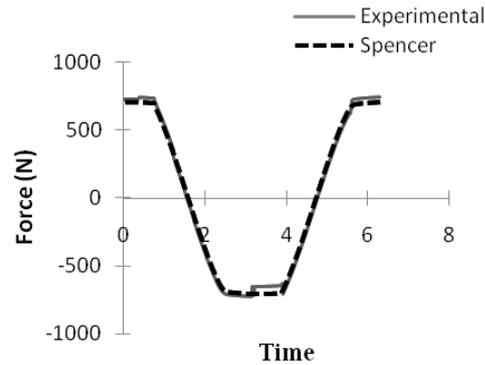
Fig. 4: Comparison of Force vs. Time of Spencer model for MATLAB/SIMULINK and Experimental analysis
