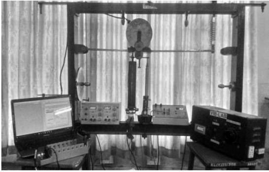
Fig. 1: Experimental setup for testing MR damper
