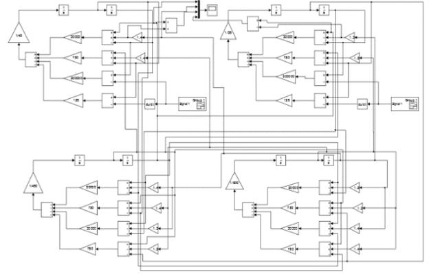
Fig. 14: Matlab/Simulink half car model for passive suspension system
