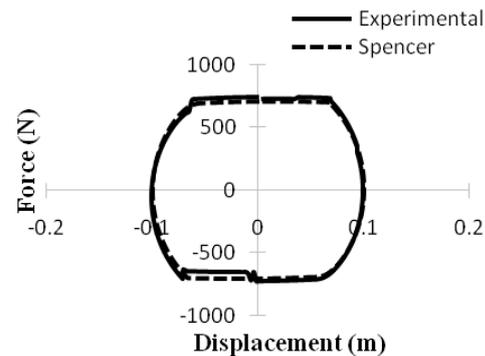
Fig. 5: Comparison of Force vs. Displacement of Spencer model for MATLAB/SIMULINK and Experimental analysis
