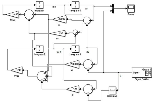
Fig. 8: MATLAB/SIMULINK model of quarter passive suspension system
