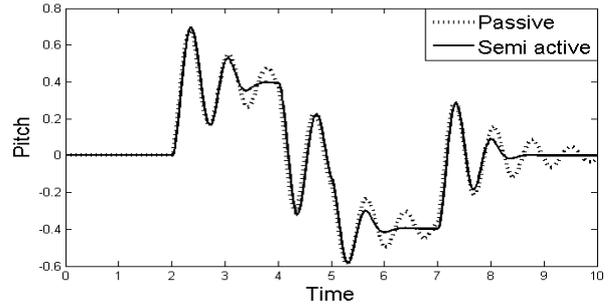
Fig. 19: Comparison of pitch for passive and semi-active half car model.
