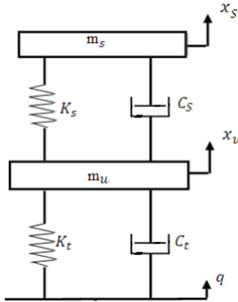
Fig. 7: Quarter car model for passive suspension system
