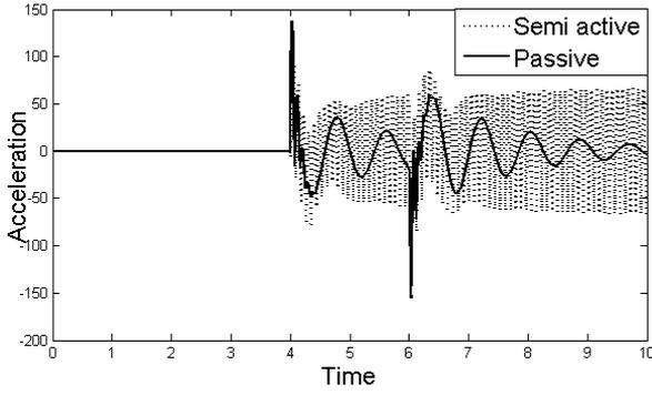
Fig. 12: Acceleration vs. Time for passive and semi-active quarter car model
