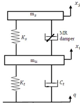
Fig. 9: Quarter car model for semi-active suspension system
