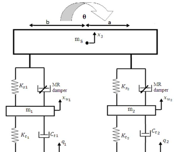
Fig. 15: Half car model for semi-active suspension system
