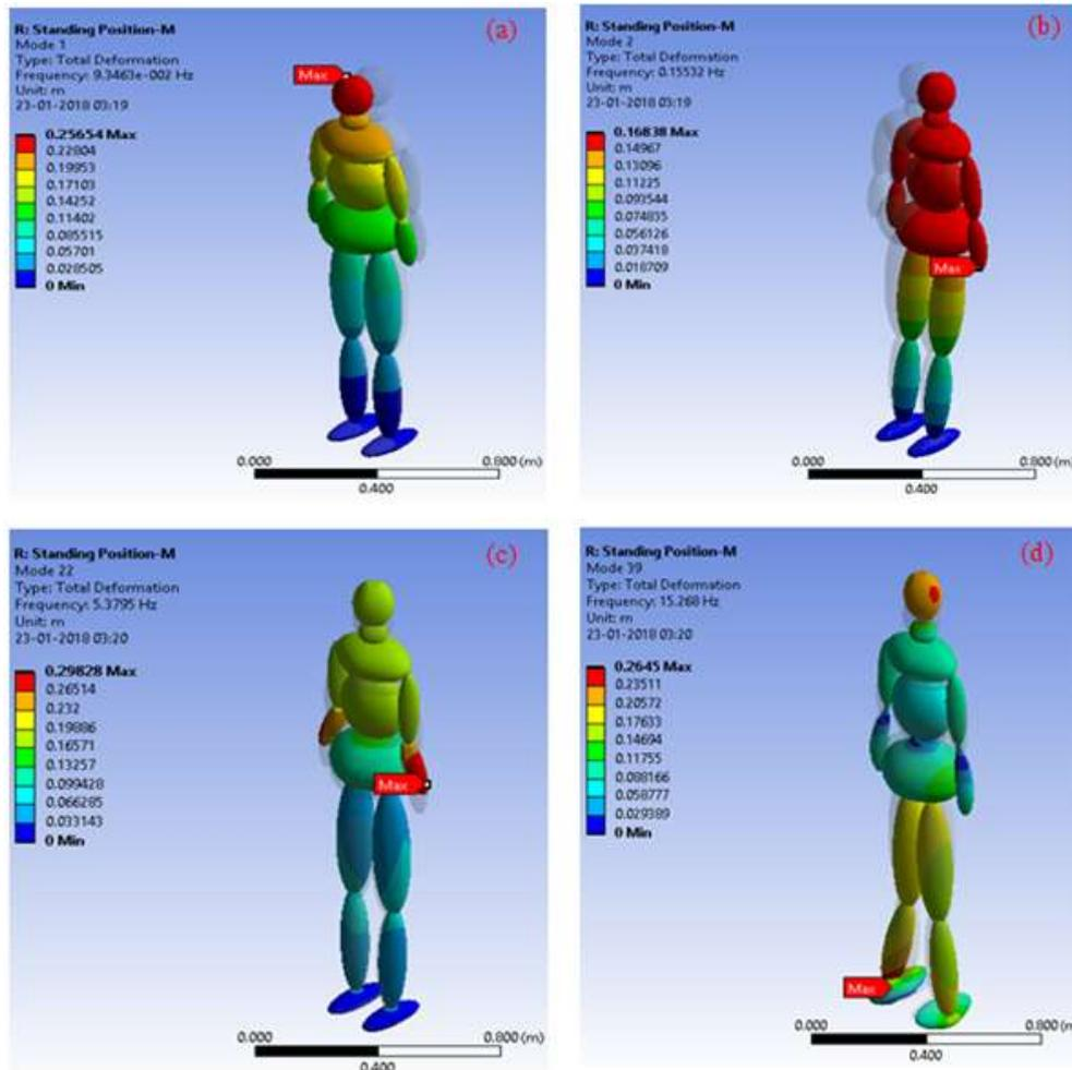
Fig. 3: Vibration modes of the model of the standing human body model. (a) First mode in the fore-and-aft direction, 0.09 Hz, (b) First mode in the lateral direction, 0.155 Hz, (c) First mode in the vertical direction, 5.3795 Hz, (d) Second mode in the vertical direction, 15.268 Hz
