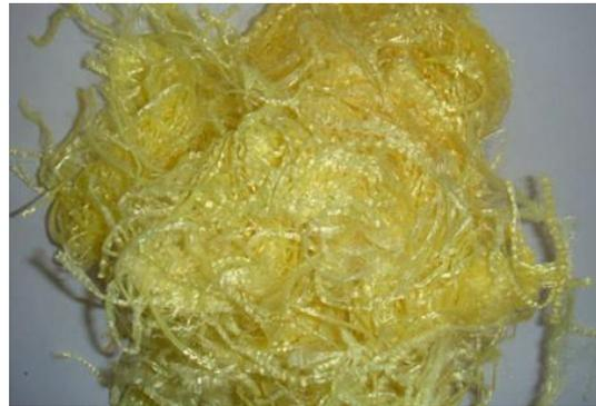
Fig. 1: Kevlar fibre
