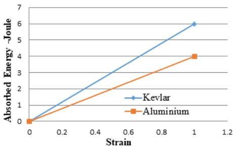
Fig. 9: Impact strength comparison of Kevlar and aluminium
