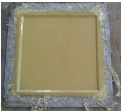
Fig. 3: Fabricated Kevlar composite material
