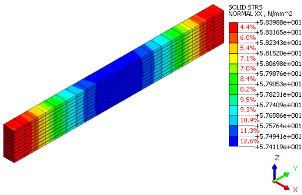
Fig. 11: Tensile stress at the resin layer (mid-span)
