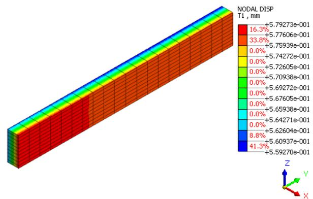
Fig. 10: Tensile elongation of Kevlar epoxy (mid-span)
