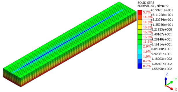
Fig. 13: Flexural stress at the resin layer (mid-span)
