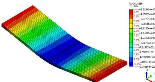
Fig. 12: Flexural displacement of Kevlar epoxy
