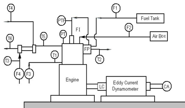
Fig. 1: Schematic setup of engine test rig
