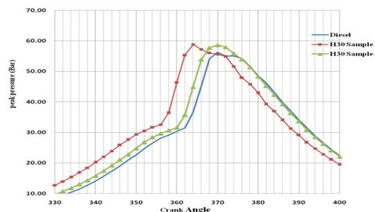
**Fig. 2: Pressure - crank angle comparison for 80% load condition**
