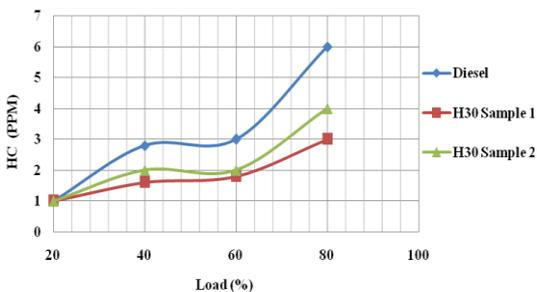
Fig. 7: HC emissions vs. Load
