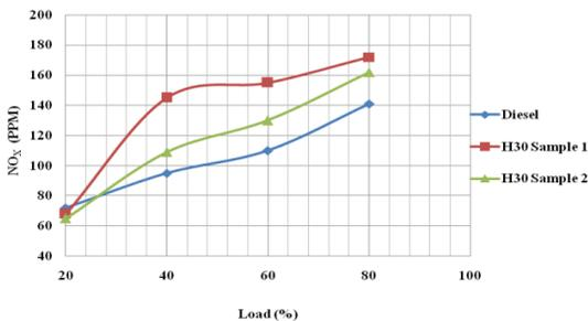
Fig. 8: NO<sub>x</sub> emissions vs. Load
