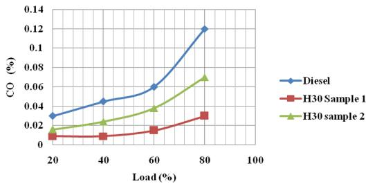
Fig. 5: CO emissions vs. Load
