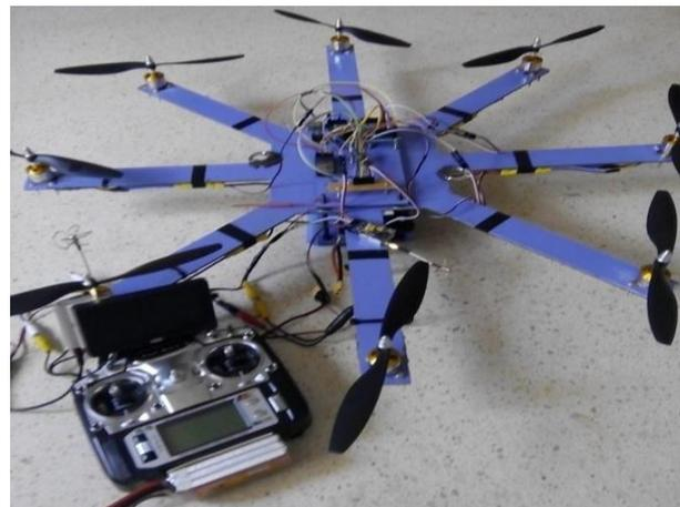
Fig. 6: Realized octocopter prototype
