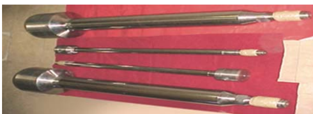
Fig. 6 — Coated spindle valves for power generating steam turbines
