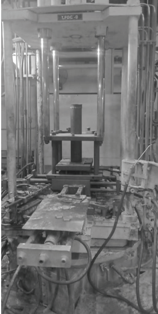
Fig.1: Experimental setup showing low-pressure die casting machine
