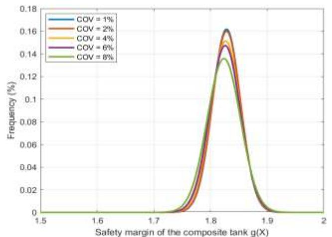
Figure 3. Safety margin distribution in terms of the different COVs of the composite tank elastic constants.
