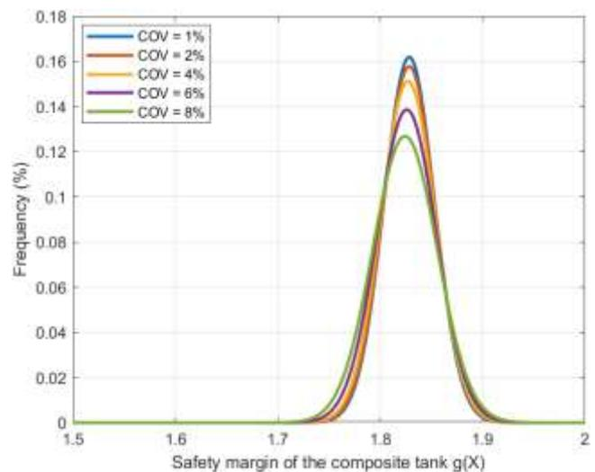
Figure 7. Safety margin distribution in terms of the different COVs of the radius of the composite tank
