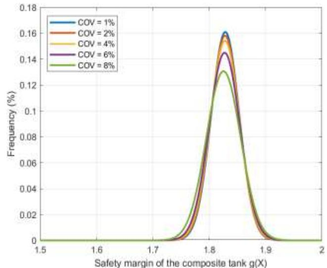
Figure 6. Safety margin distribution in terms of the different COVs of the thickness of the composite tank
