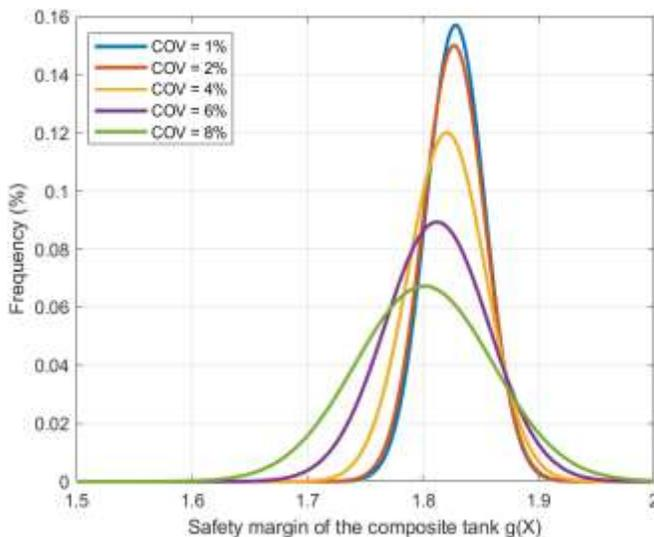
Figure 5. Safety margin distribution in terms of the different COVs of the winding angle of the composite tank
