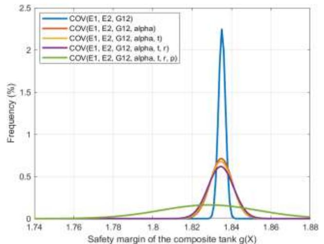
Figure 2. Safety margin distribution in terms of the different cylindrical composite tank uncertainties.
