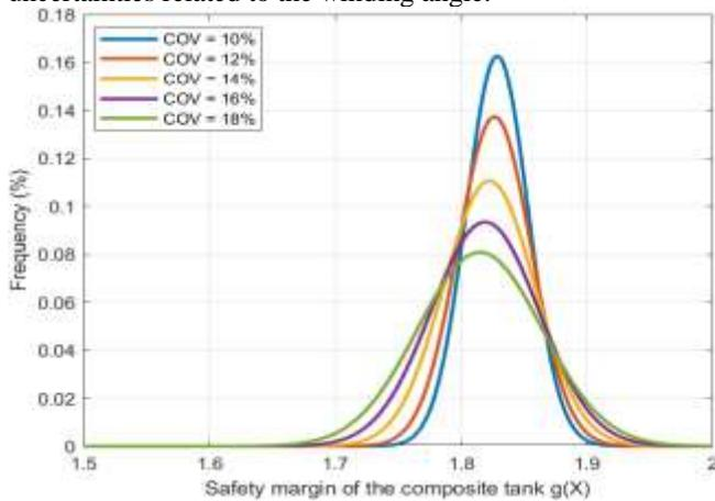
Figure 4. Safety margin distribution in terms of the different COVs of the internal pressure of the composite tank
