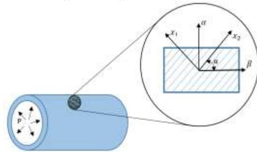
Figure 1. Relation of coordinate system between local axes and principal material axes.
