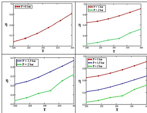
**Figure 12.** Variation of the yield as a function of the temperatures for different low pressures ( $P_H = 10$  bar)
