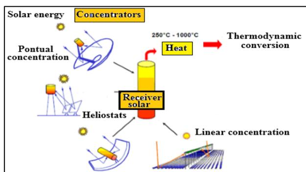
**Figure 3.** Global diagram of the solar-thermal conversion
