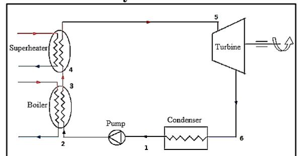
Figure 9. Schematic diagram of the HIRN cycle
