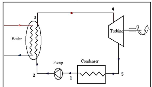
**Figure 7.** Schematic diagram of the RANKINE cycle
