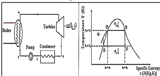
**Figure 5.** Schematic diagram of the RANKINE cycle
