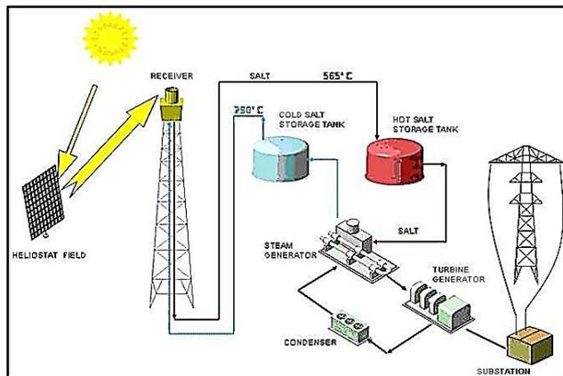
**Figure 1.** Schematic diagram of a concentrated solar power station
