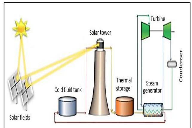
**Figure 2.** Principle of operation of a concentrated solar thermal power station [17]
