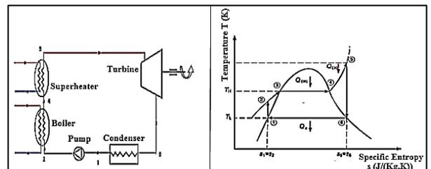
**Figure 6.** Schematic diagram of the HIRN cycle
