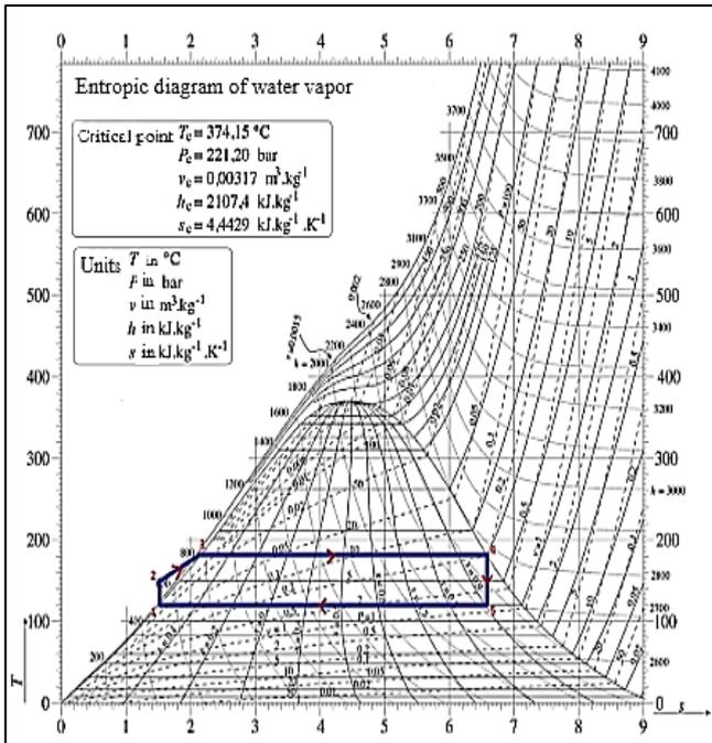
Figure 8. RANKINE cycle between 2 and 10 bar
