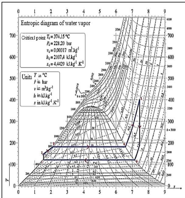
**Figure 10.** HIRN cycle between 2 and 10 bar at 400 ° C
