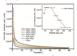
Fig. 5 — Particle size effect on NaLi<sub>2</sub>PO<sub>4</sub>:Cu<sup>2+</sup> irradiated at Υ-ray Co<sup>60</sup> source.
