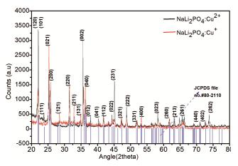
Fig. 1 — XRD form of the NaLi<sub>2</sub>PO<sub>4</sub> phosphors (our material). The data available in the literature" JCPDS File# 80-2110" is also given for comparison.
