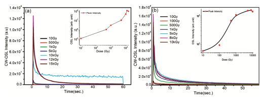
Fig. 6 — (a) OSL Dose response curve (ranging from 10Gy-15kGy) of  $\text{NaLi}_2\text{PO}_4$ :Cu<sup>2+</sup> stimulated by the blue LED (80mW,470nm) before irradiation the 0.1mol% phosphor material annealed at 1073K for 1.0 h, (b) OSL Dose response curve (ranging from 10Gy-8kGy) of  $\text{NaLi}_2\text{PO}_4$ : Cu<sup>+</sup> stimulated by using blue LED (470nm, 80mW). The phosphor was annealed at 873K for 1h before irradiation with 0.08 mol%.
