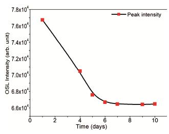
Fig. 9 — Typical CW-OSL decay curves of NaLi<sub>2</sub>PO<sub>4</sub>:Cu<sup>2+</sup> taken 1.0hr after irradiation and storing in dark at room temperature (300K). Fading was taken starting from the same day up to 10 days.
