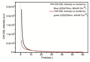
Fig. 4 — Effect of the stimulation source on the CW-OSL decay curves of NaLi<sub>2</sub>PO<sub>4</sub>:Cu<sup>2+</sup> stimulation by Blue LED (80mWcm<sup>-2</sup>) and green LED (80mWcm<sup>-2</sup>). The material was irradiated at 10Gy of Y- ray Co<sup>60</sup> source.
