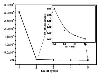
Fig. 8 —  $Cu^{2+}$  doped  $NaLi_2PO_4$  Readouts many times irradiated with 10 Gy  $Co^{60}$  Y-source. Shows OSL Intensity v/s no. of cycles. It is seen from Fig. 8 that during first readouts, more than 50% intensity was vanished. An expanded view of the successive readouts is shown in the inset of the figure.
