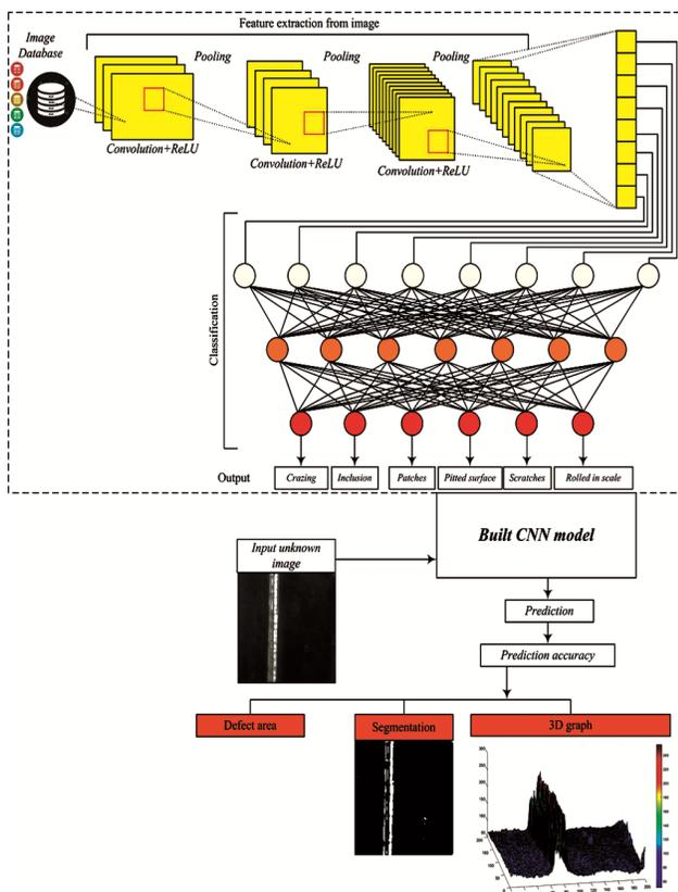
Fig. 1 — The architecture of the CNN
