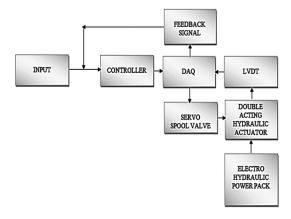
Fig. 1 — Block diagram of EHSS
