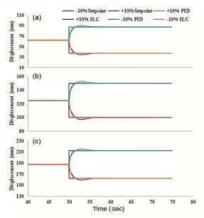
Fig. 7 — Simulation result of servo response at: (a) 62.5 mm, (b) 125 mm, (c) 187.5 mm
