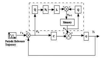
Fig. 4 — Block diagram of iterative learning controller
