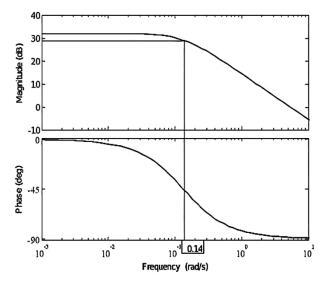
Fig. 5 — Magnitude and Phase of Bode plot
