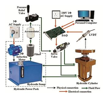
Fig. 3 — Functional flow diagram of EHSS
