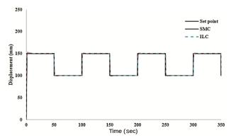
Fig. 12 — Simulation result of square wave response of ILC and SMC at 50% of pulse width
