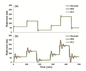
Fig. 11 — Set point tracking: (a) simulation result, (b) experimental result
