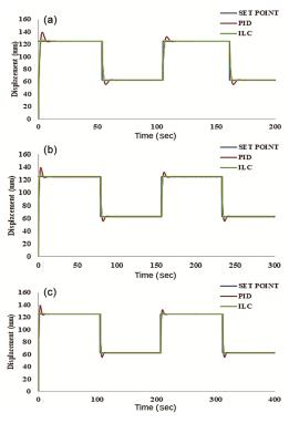
Fig. 9 — Simulation result of square wave response at: (a) 50% of pulse width, (b) 75% of pulse width, (c) 100% of pulse width
