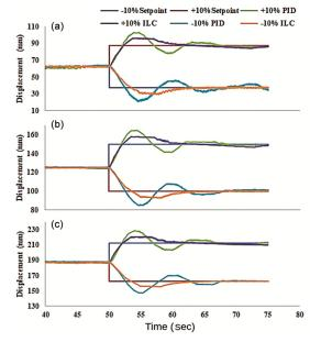
Fig. 8 — Experimental result of servo response at: (a) 62.5 mm, (b) 125 mm, (c) 187.5 mm
