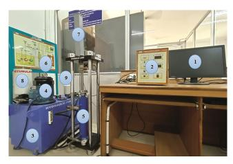
Fig. 2 — Photography of EHSS: 1-Personal computer (PC), 2-DAQ, 3-Hydraulic power pack, 4-Three phase fixed displacement pump, 5-Double-acting hydraulic cylinder, 6-Pressure gauge, 7-LVDT, 8-Accumulator, 9-Servo spool valve
