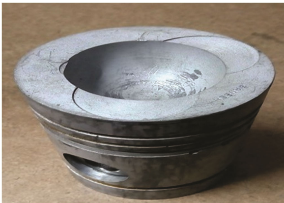
Fig. 2 — Photographic view of lanthanum aluminate-coated surfaces of the cylinder piston
